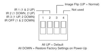
A label on the bottom of the camera provides a quick reference for setting the DIP switches.
