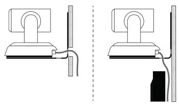
4. Attach the camera to the mount using the mounting screw supplied with the camera.
